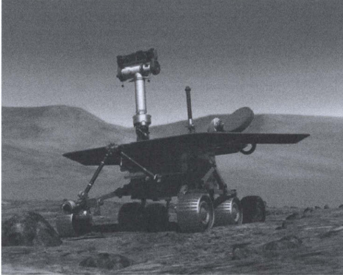
Figure 1.11. An artist's impression of the rover Spirit on the surface of Mars. The robotic arm used to position scientific instruments is clearly visible. Image reproduced courtesy of NASA/JPL-Caltech.
